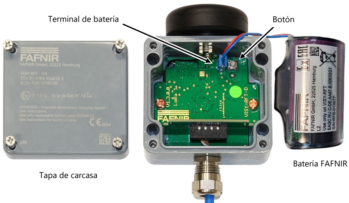
Figura 14: Transmisor VISY-RFT; vista interior
