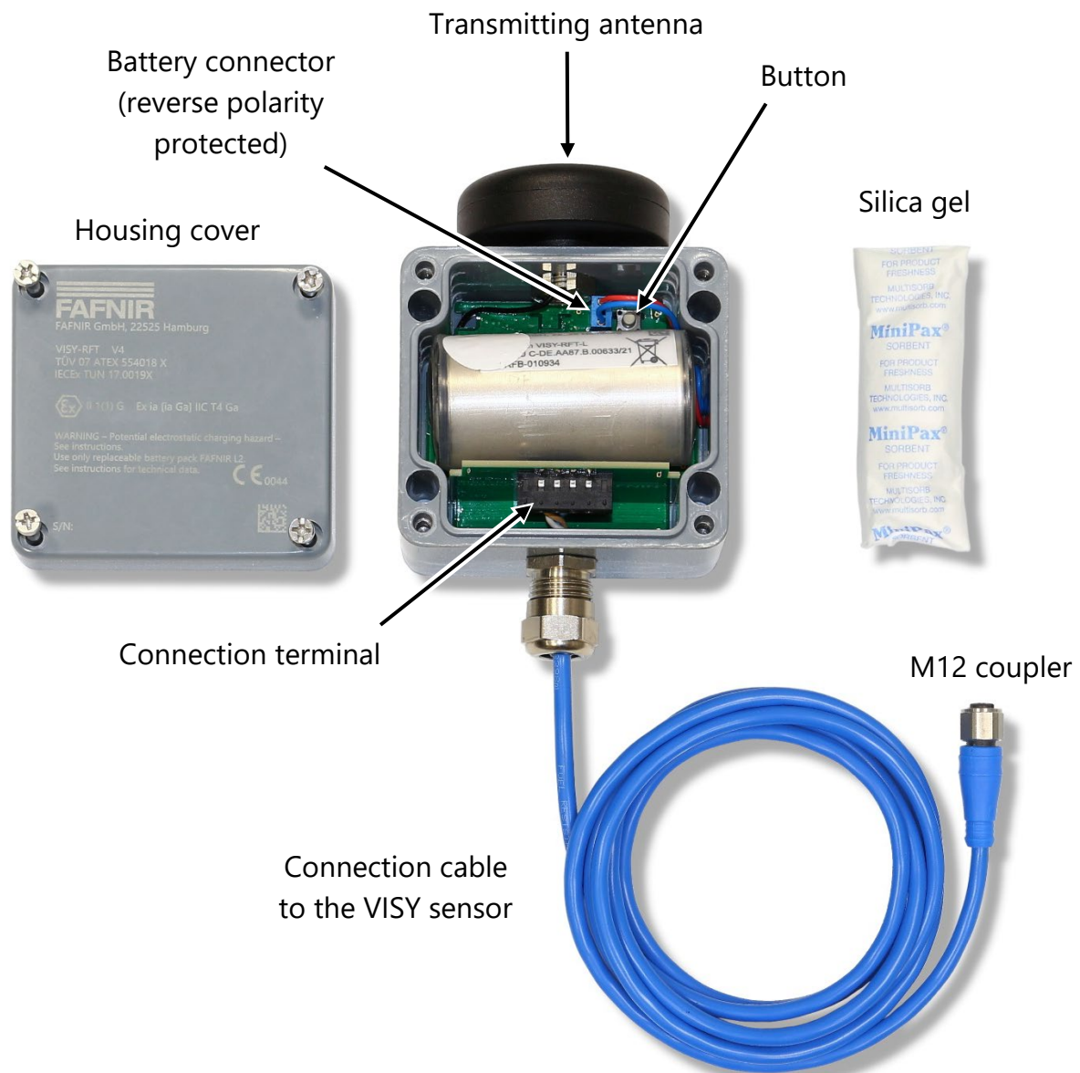
Figure 1: VISY-RFT V4 transmitter with cover removed
