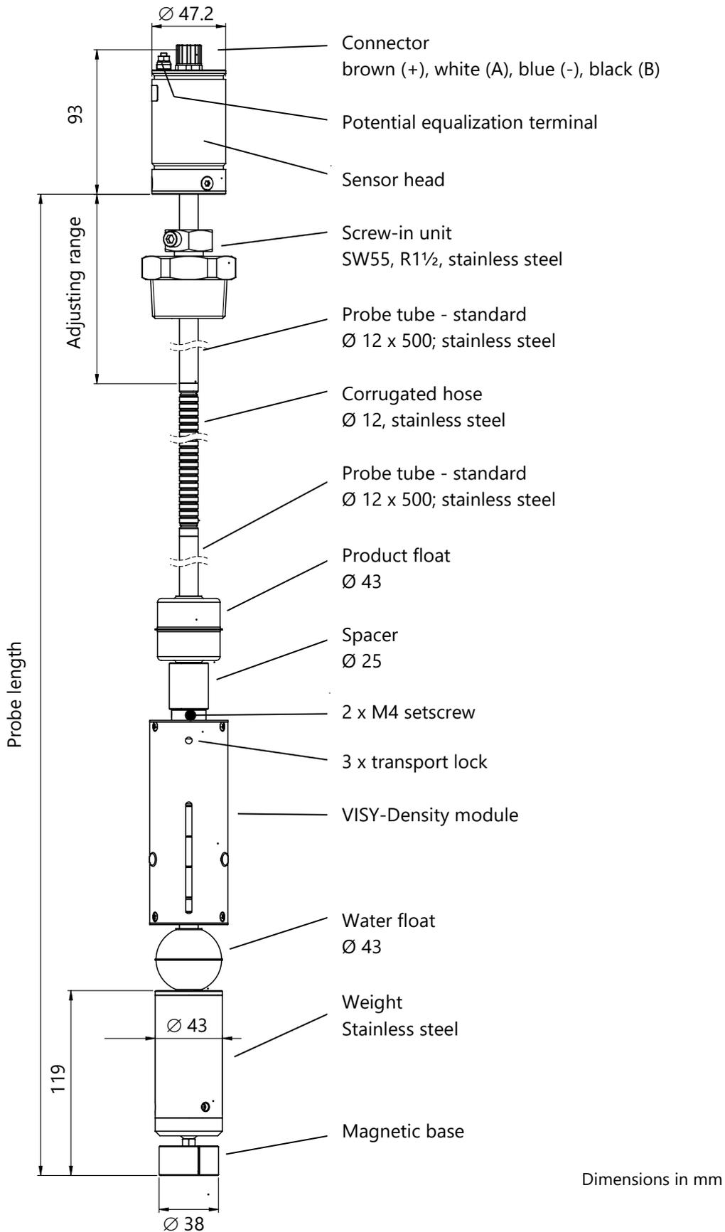
Figure 5: VISY-Stick Flex with VISY-Density Module
