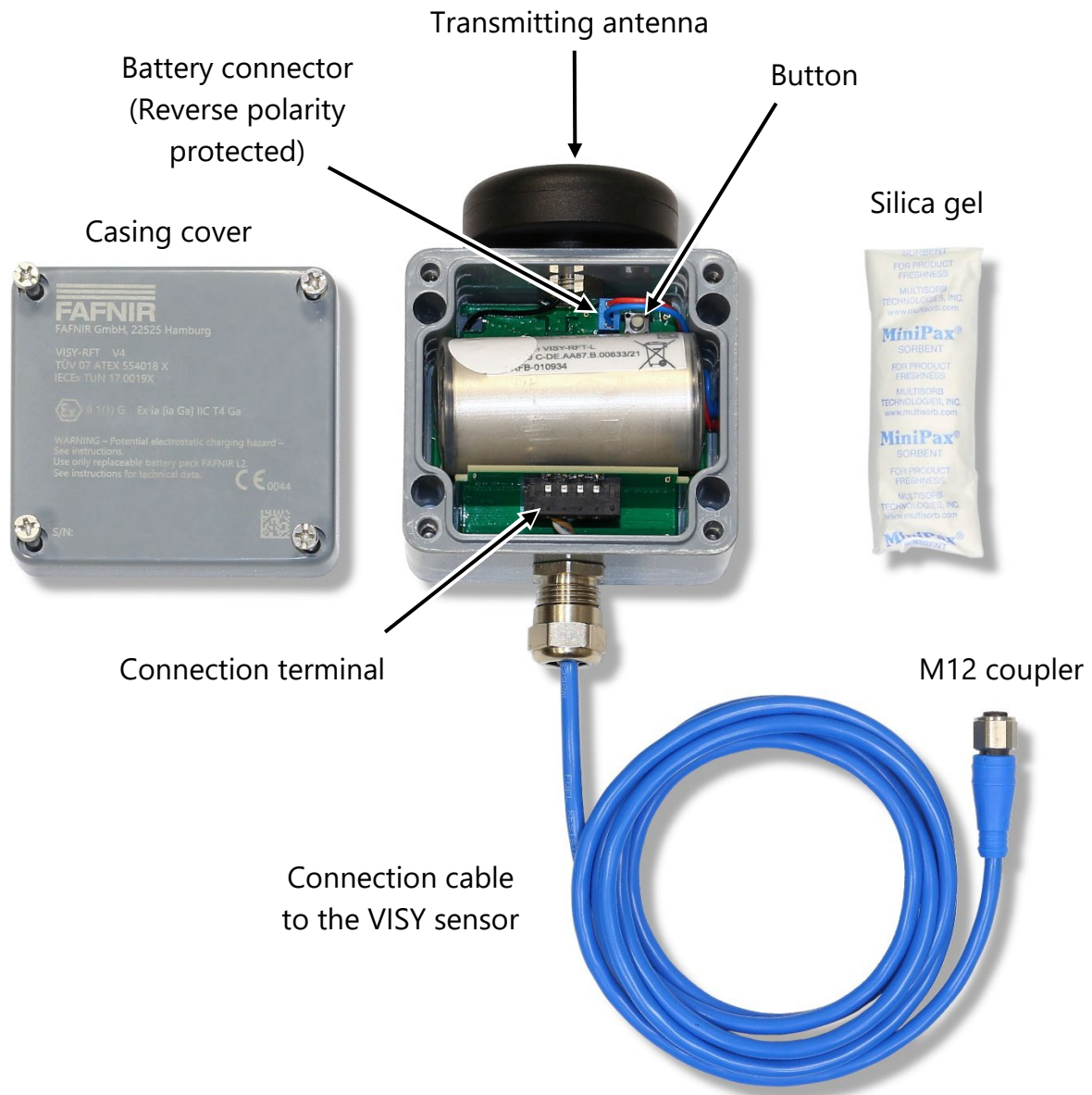
Figure 1: VISY-RFT V4 transmitter with cover removed
