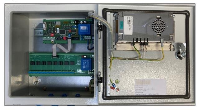
All cables must be secured so that they cannot lie on or fall onto the VP board.
