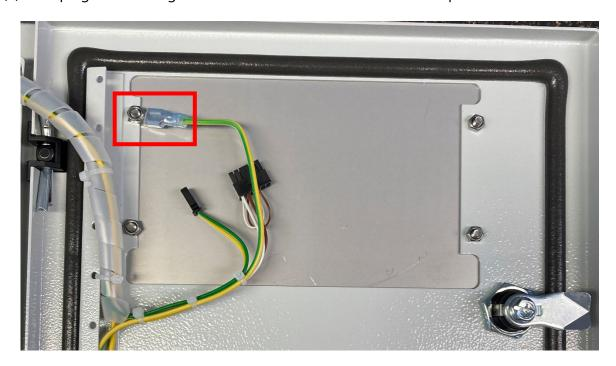
(2) Remove the 4 nuts from the backside of the plate and remove the plate completely from the VISY-Command GUI.
