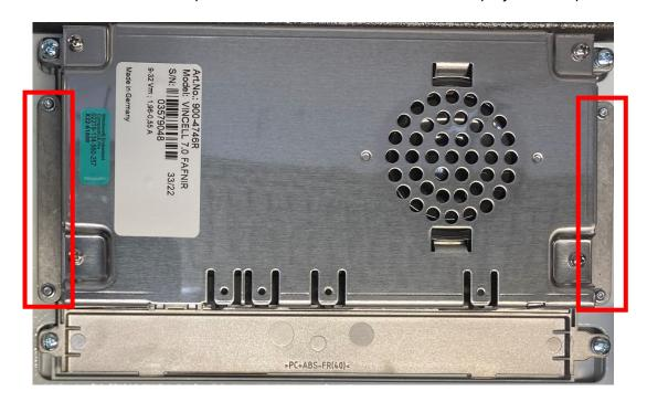
(2) Carefully insert the new display into the VISY-Command GUI door and align it properly with the door. Now place the 2 metal rods plates on either side of the display and screw them onto the door so that the display is fixed to the door.
