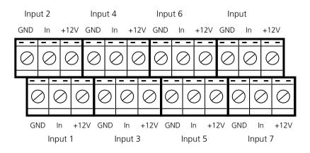
Figure 3: Screw terminal inputs
