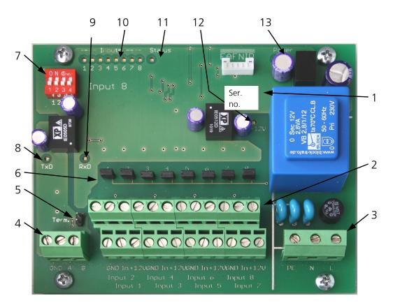
Figure 1: VISY-Input Design
