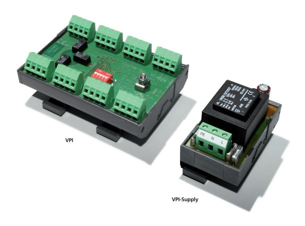
The VPI (VISY-Power Interface) provides a communications interface between the sensors and a higher-level system (master). For the sending of commands to the sensors, the VPI supports two protocols\*. The response is assigned and forwarded to the individual sensor terminals.
