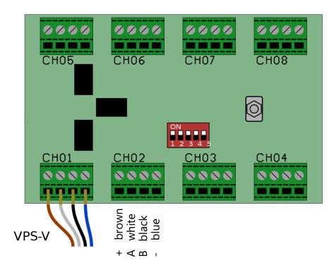
Figure 5: Connectors of VPI measuring transducer
