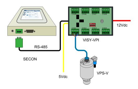
Figure 4: Wiring of the VPS-V pressure sensor to the SECON
