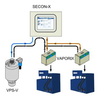
Figure 2: VPS-V pressure sensor as part of the vapour recovery monitoring system
