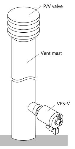
Figure 3: Mounting on the vent mast
