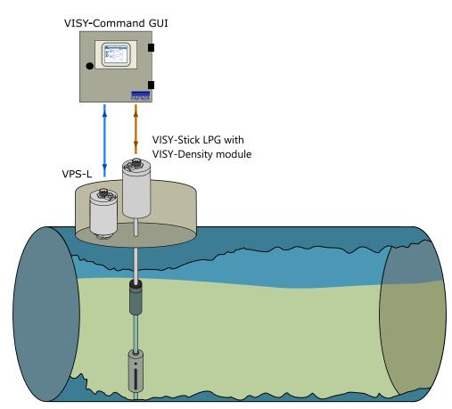
Figure 6: VPS-L pressure sensor for monitoring the vapour pressure in LPG tanks
