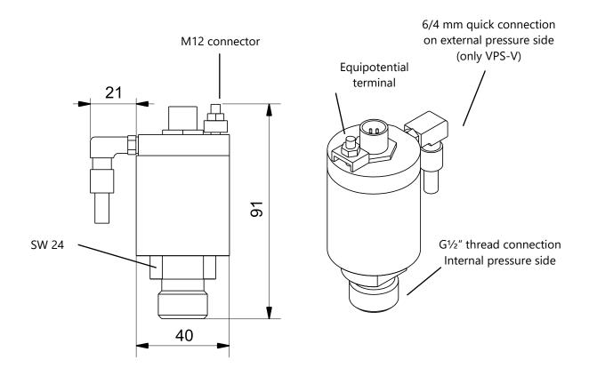
Figure 1: Dimensions of VPS-V pressure sensor
