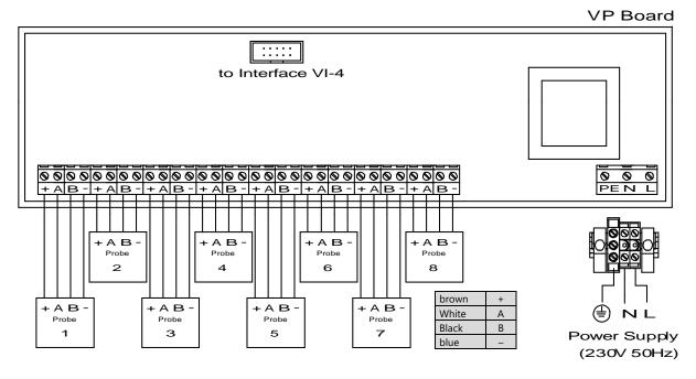
Figure 8: Connection of VPS-L pressure sensor to the VP board in VISY-Command
