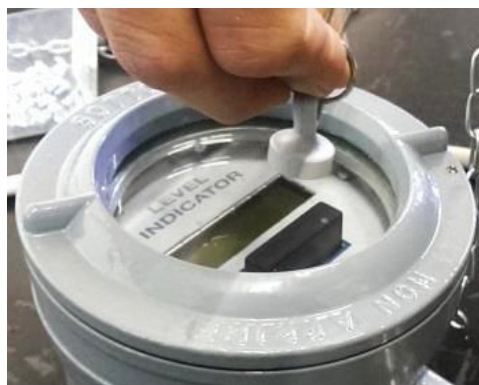
Figure 2: Operation with the aid of the magnet
