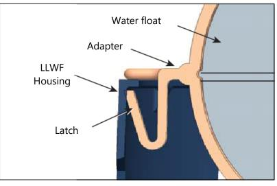
Figure 3: Correct Adapter Latch Position Under LLWF Housing Flange
