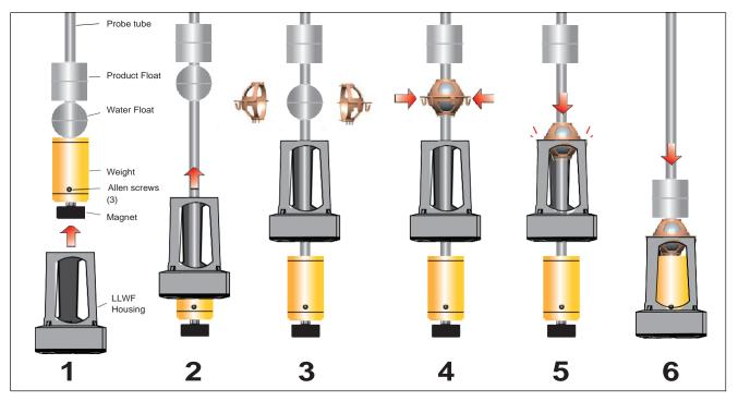
Figure 2: Mounting the LLWF kit
