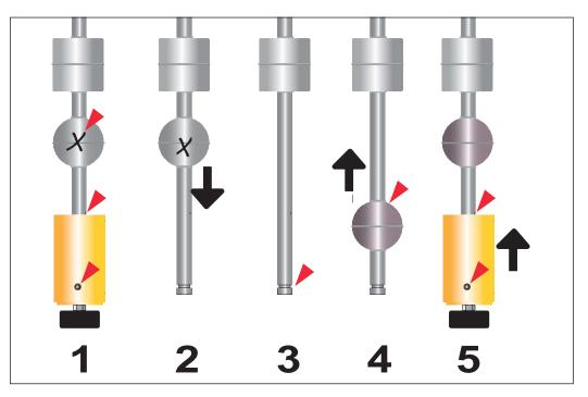
Figure 5: Install the Replacement Water Float
