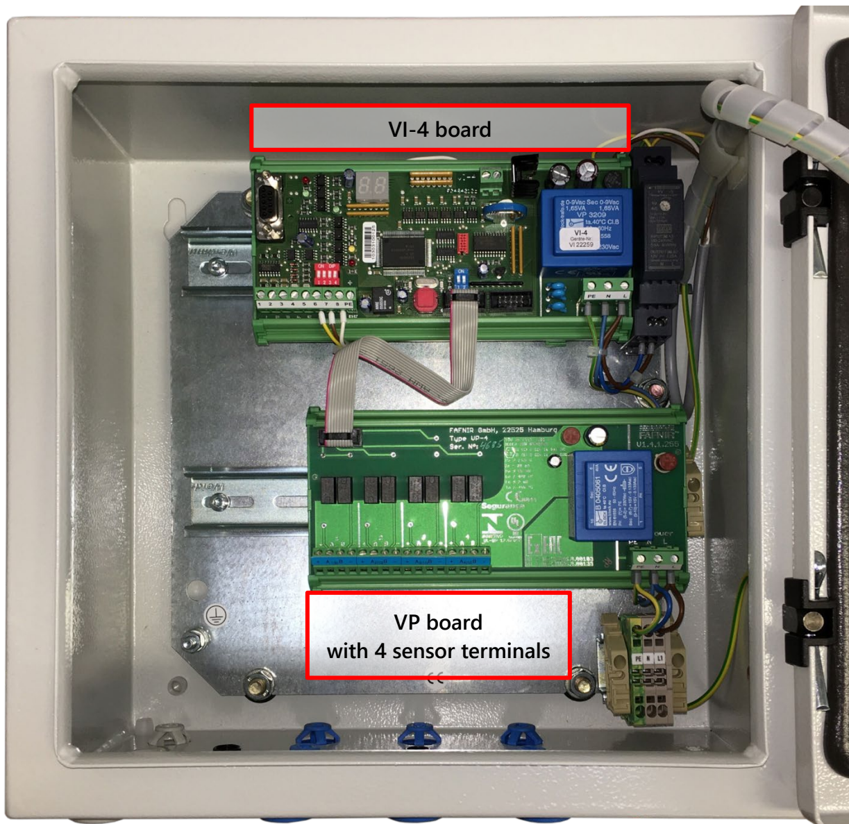
Figure 2: VISY-Command 4 GUI, interior view
