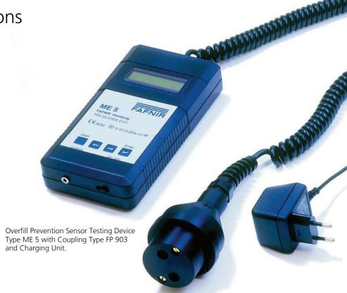
Since the overfill prevention sensor testing device type ME 5 has its own instrinsically safe output circuit it can be used for testing all overfill prevention sensor testing devices certified as per TRbF (also the ones applied in zone O). The ME 5 itself has to be operated outside the ex-zone. The coupling type 903 required for connecting the GWG is equipped with the corresponding cable length.
