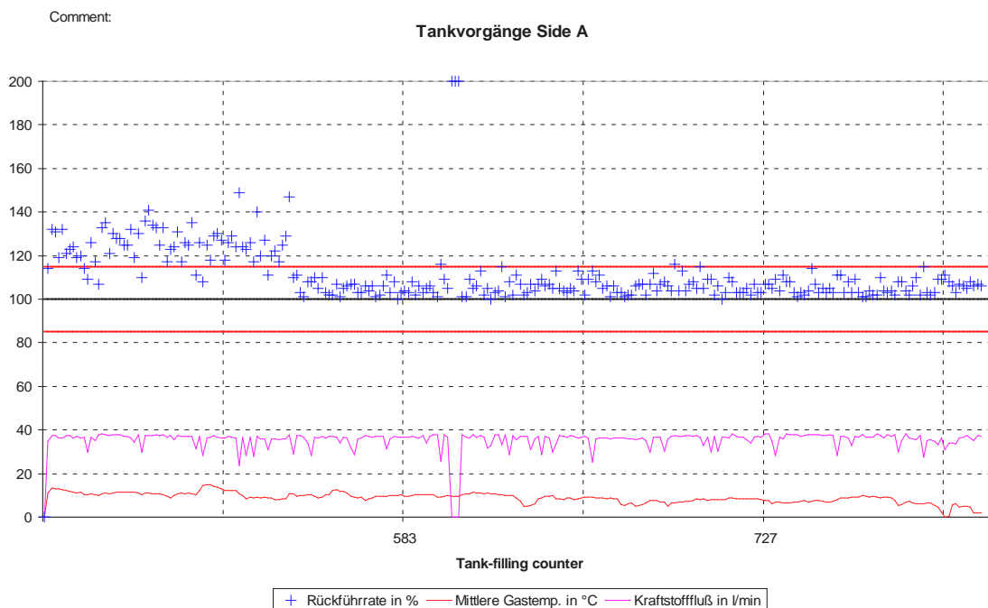
Figure 20: Speed-controlled vapour recovery system with diaphragm pump and too short pipe connection between VAPORIX-Flow and the pump. During refuelling operation 520, a pulsation damper was installed. The recovery rates and the spread of the measurement values decreased considerably.
