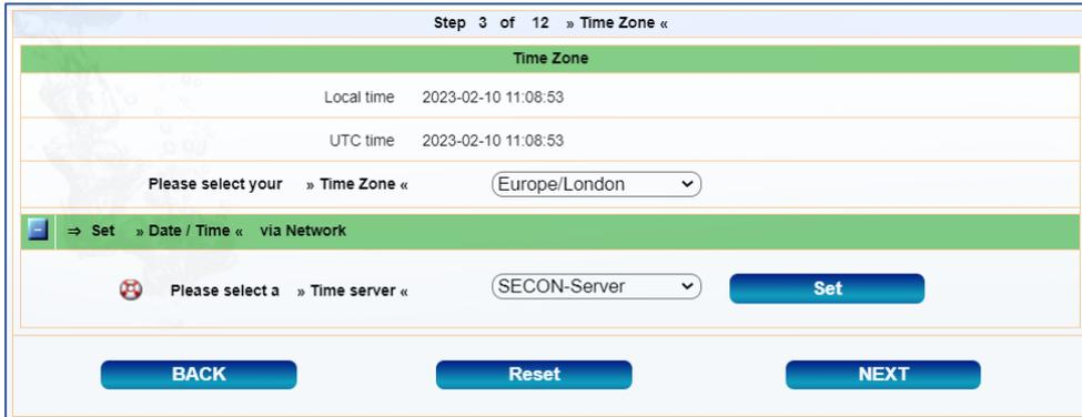
Date and time of the **SECON-Client** devices are synchronized with a time server. If no connection to the SECON-Server shall be established, another server can be selected here, e.g. "de.pool.ntp.org" for Germany.
