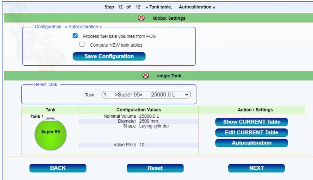
**Global Settings** in the top section: Activating (click on) the checkbox "**Process fuel sale volumes from POS**" starts the autocalibration, deactivating the checkbox stops the autocalibration. With the "**Compute new tank tables**" option, new tank tables are calculated once a day for each tank using the data from the POS. The **<Save configuration>** button saves the current settings for the autocalibration.
