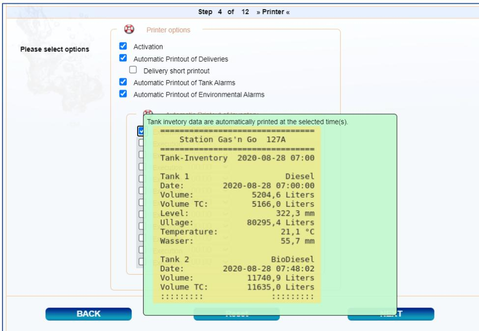
The built in printer of the VISY-Command Web can be activated here for printouts in the event of deliveries, alarms or daily reports at freely selectable times.
