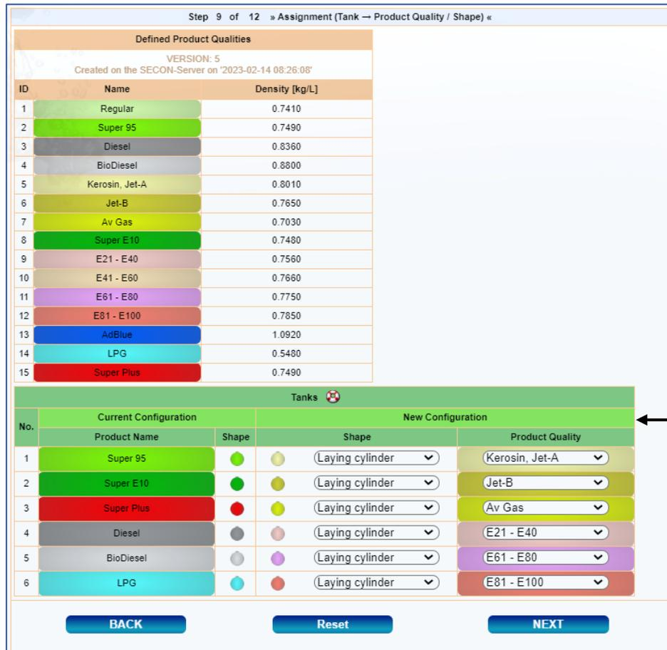
The screenshot shows the 'Assignment (Tank → Product Quality / Shape)' screen. The top section, 'Defined Product Qualities', lists 15 product types with their densities. The bottom section, 'Tanks', is split into 'Current Configuration' and 'New Configuration'. An arrow points to the 'New Configuration' section, which shows tanks 1 through 6 with their current and new product names and shapes.
