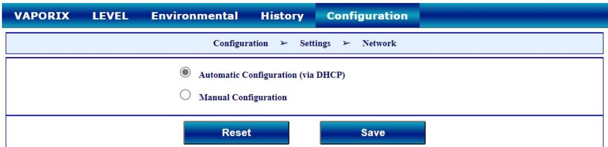
The network can be configured automatically. With this configuration, the client requests the IP address from the DHCP server directly. A functional DHCP server must be available in the network for this. For this, select the option "Automatic configuration" and confirm by pressing the <Save> button.
