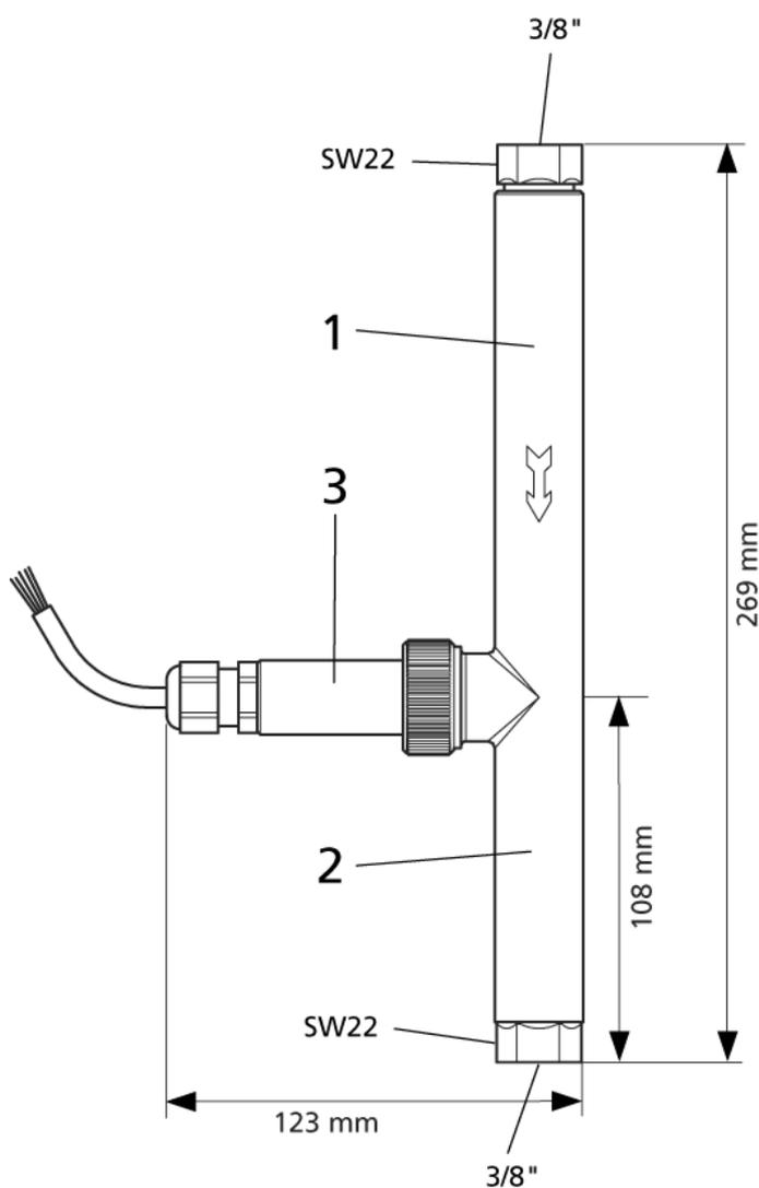
Figura 1: Sensor VAPORIX-Flow
