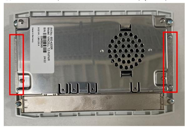
(2) Carefully insert the new display into the VISY-Command Web door and align it properly with the door. Now place the 2 metal rods plates on either side of the display and screw them onto the door so that the display is fixed on the door.
