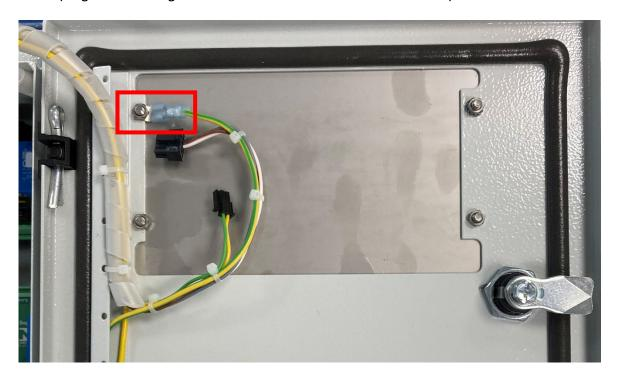
(2) Remove the 4 nuts from the backside of the plate and remove the plate completely from the VISY-Command Web.
