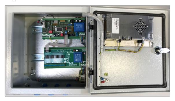
All cables must be secured so that they cannot lie on or fall onto the VP board.
