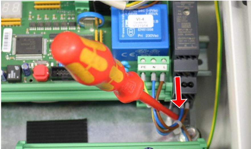
Figure 4: 12 V Power supply unit, spring clip
