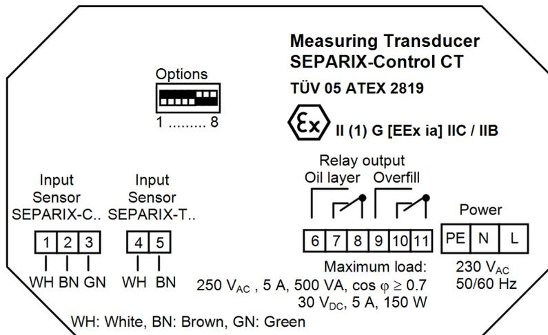
Figure 6: SEPARIX-Control CT, terminals and "Options" DIP switch
