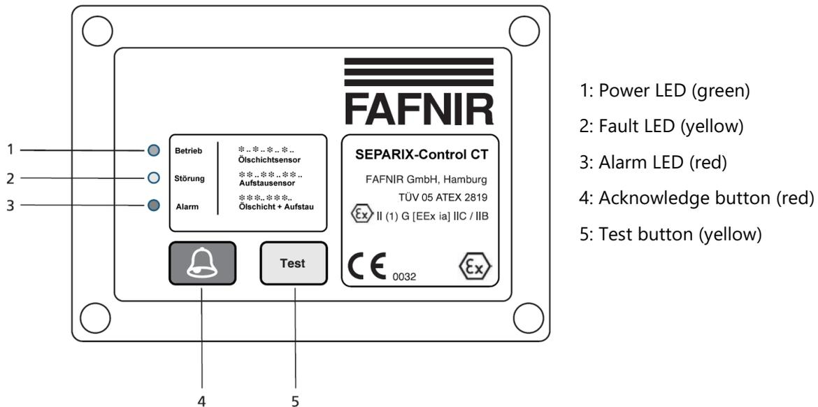
Figure 7: SEPARIX-Control CT, fault and alarm display
