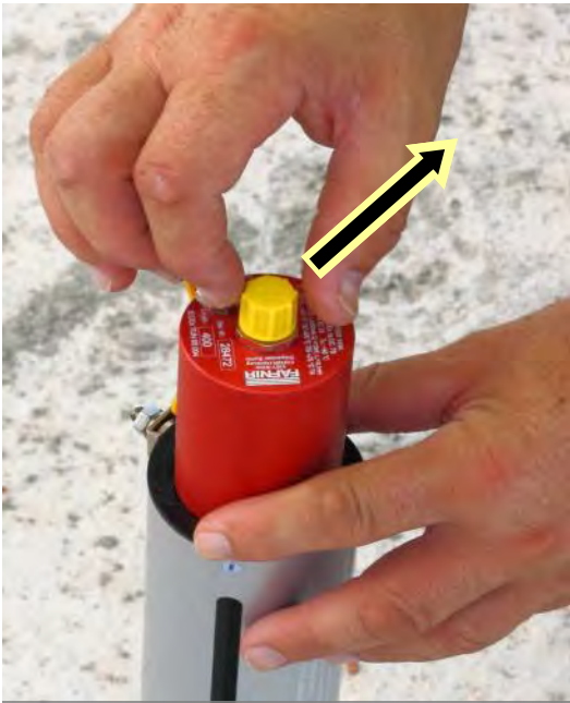
Unscrew yellow cap and connect the plug
