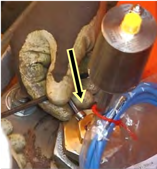
Fix the locking screw with hexagon socket key
