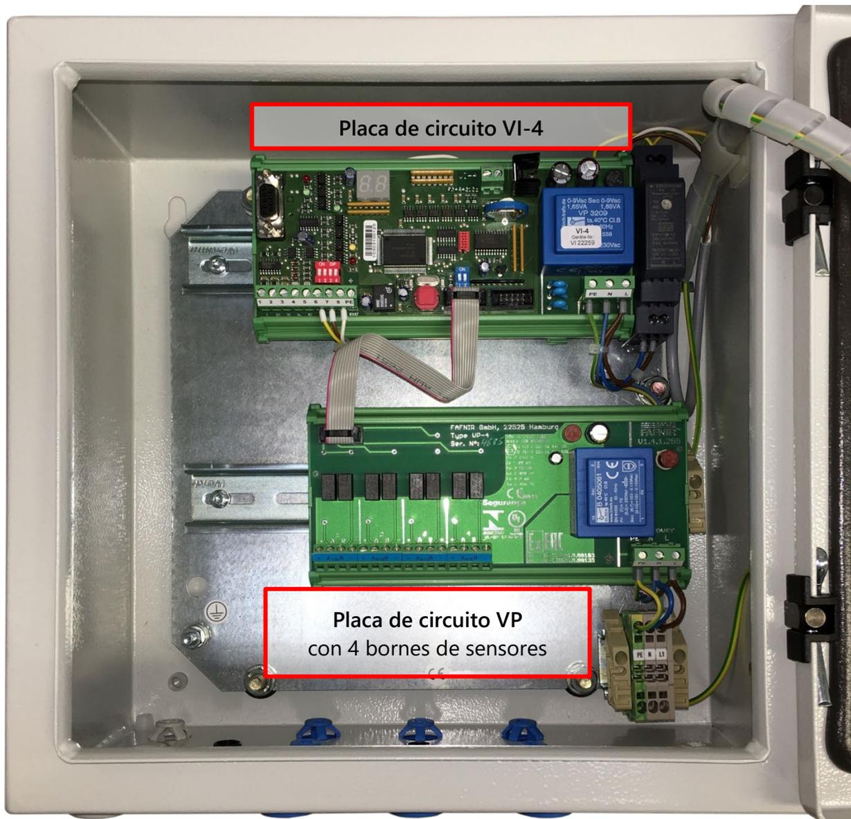
Figura 2: VISY-Command 4 GUI, vista interior
