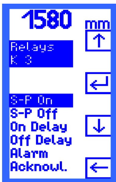
Figura 14: Pantalla Relays K1 ... K5
