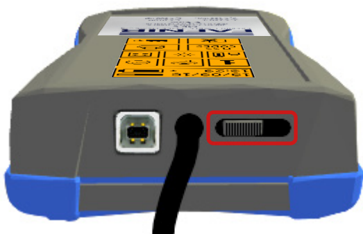
Figure 28: Switch in USB position (charging position)
