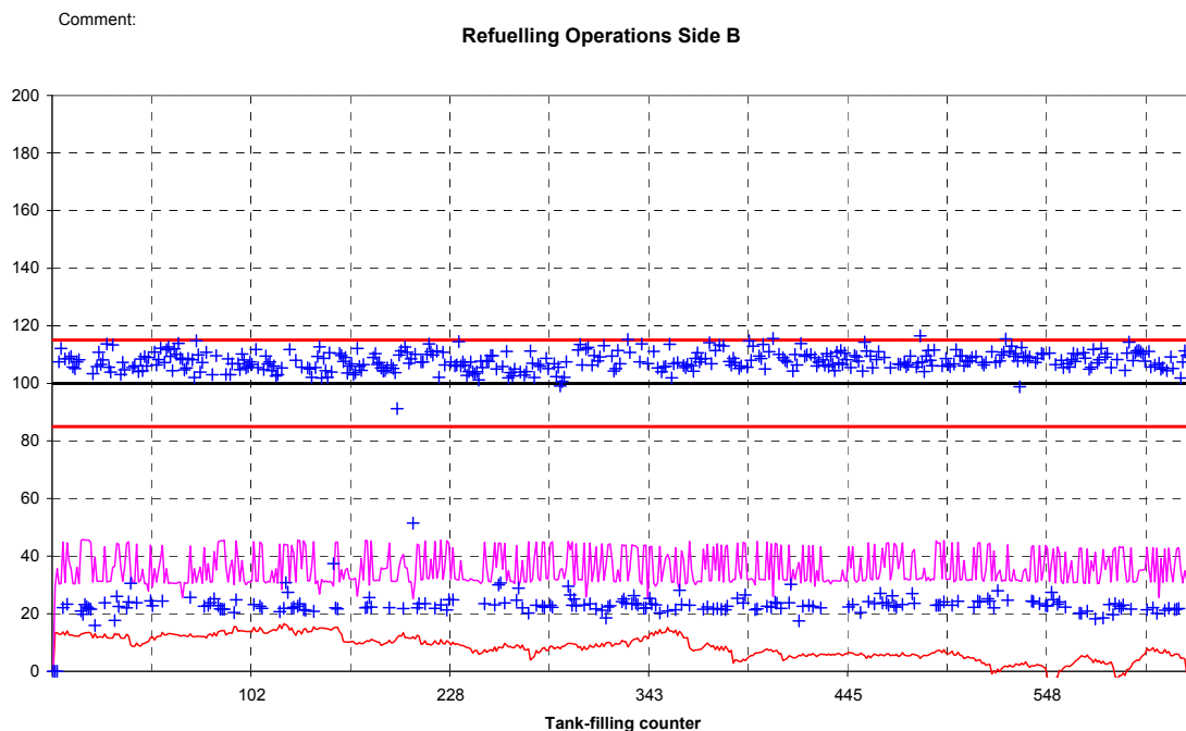
Figure 7: MPD with one incompletely opening Open/Close valve. Some of the refuelling operations exhibit a recovery rate of only 25%.
