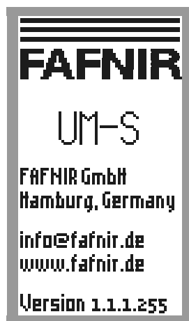
Fig. 3: The "Information" display is shown for 5 seconds after switching on the measurement analysis system
